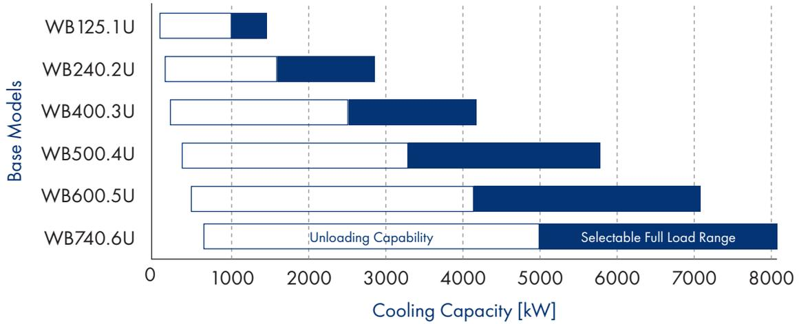
Note: Available cooling capacity will vary with operating conditions and chiller configuration. Capacities shown are based on standard AHRI conditions.
