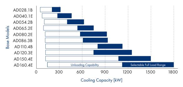
Note: Available cooling capacity will vary with operating conditions and chiller configuration. Capacities shown are based on standard AHRI conditions.
