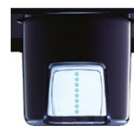
8 sensors measure while moving left to right
